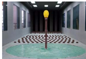
Luo, Y. & Wang, Yucheng & Xie, J. & Yang, C. & Zheng, Yanfeng. (2017). Aero-elastic wind tunnel test of a high lighting pole. Wind and Structures, An International Journal . 25. 1-24.
