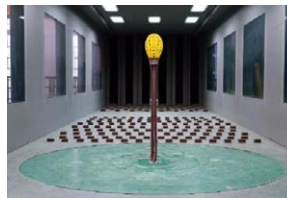
Luo, Y. & Wang, Yucheng & Xie, J. & Yang, C. & Zheng, Yanfeng. (2017). Aero-elastic wind tunnel test of a high lighting pole. Wind and Structures, An International Journal . 25. 1-24.
